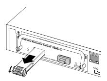
Figure 18: Removing an XFP Module
